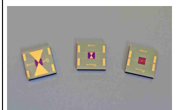
Bow-tie antennas with different geometrical parameters
